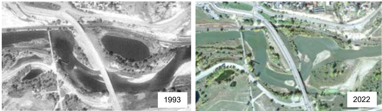
Figure 6-9. Gravel pond upstream of bridge at Rifle, Colorado captured by the Colorado River.
