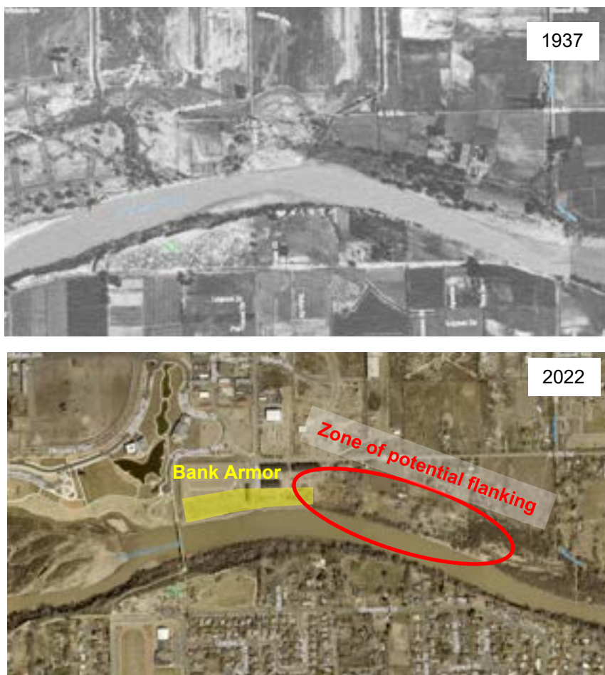
Figure 6-15. Bank armoring east of Las Colonias that ends at apex of outer meander bend may be subject to flanking by channel migration.
