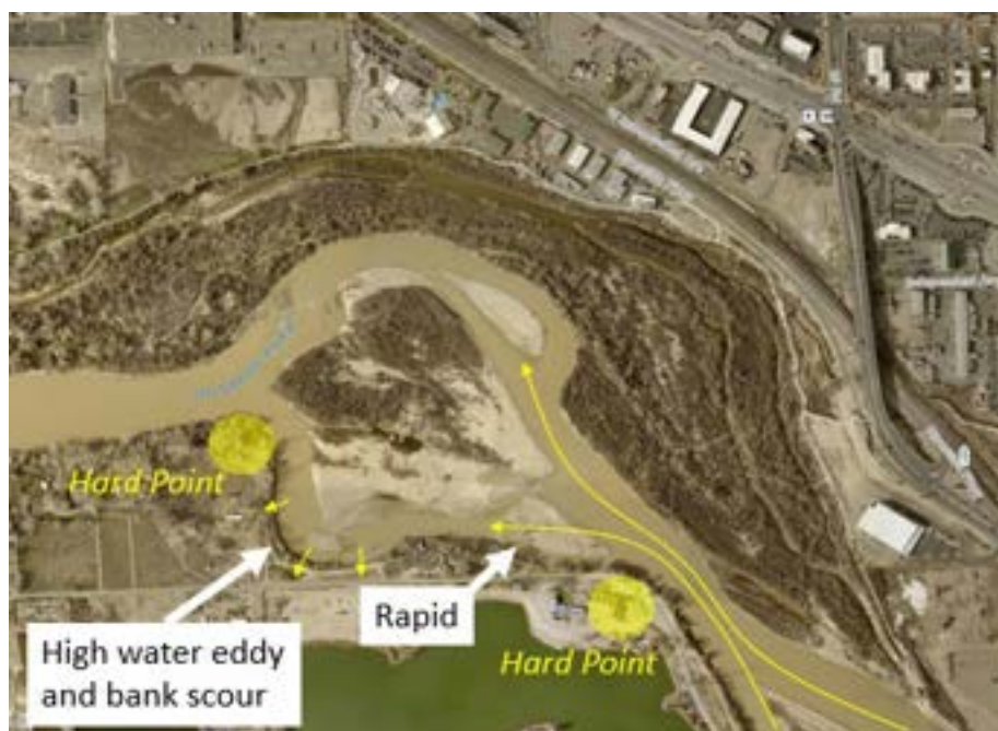
Figure 6-18. Arrested down valley channel migration and artificially forces southward migration at Dike Road near Connected Lakes State Park.
