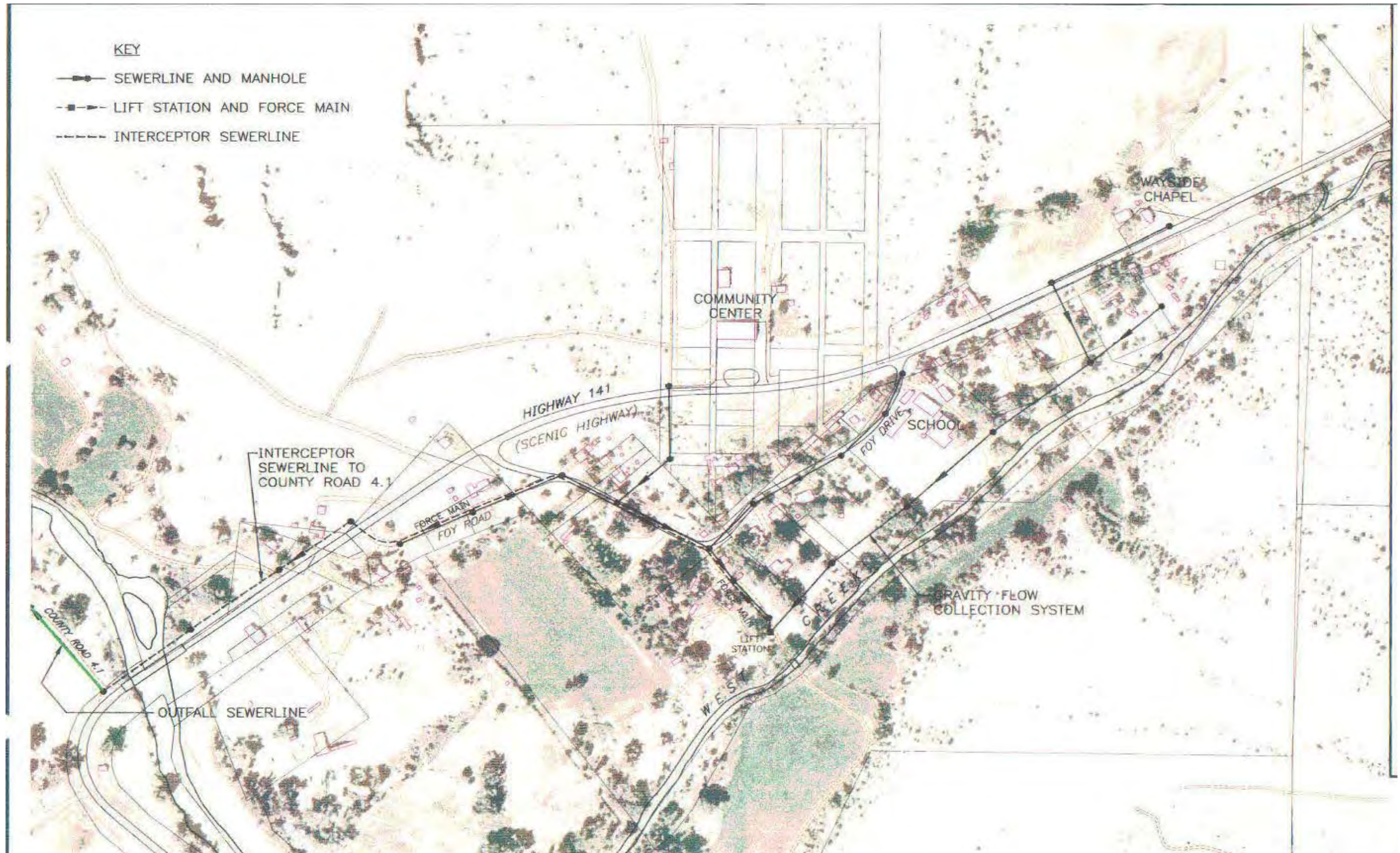
Figure 2 Preliminary Sewer Line Configuration
