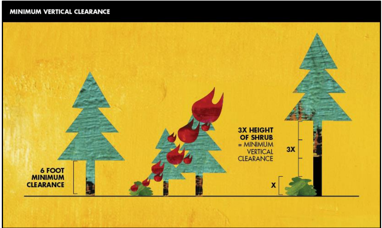
Figure F.3. Recommended minimal vertical clearance.
